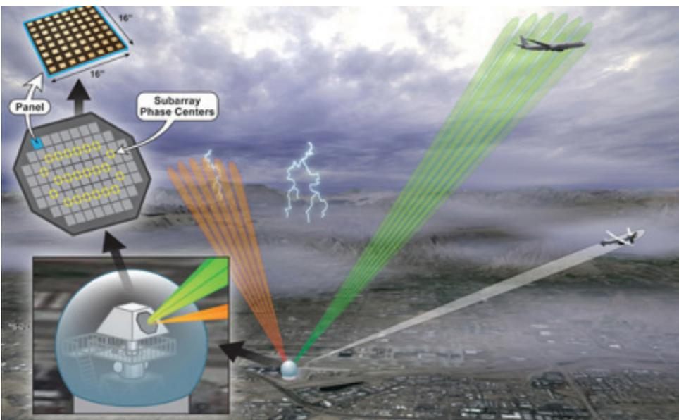
Aviation MPAR concept of operations with tilted four face fixed array (Courtesy of Lincoln Labs)
