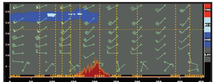
Vertical cross-section of wind speed and turbulence intensity along a user selected flight route.
