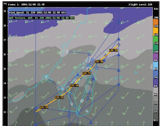
Plan view graphic of the winds at flight level 220 and along a user defined route of flight. Wind speed is color coded and the user selected flight route is highlighted.
