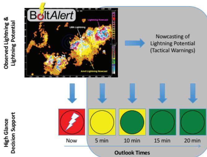
BoltAlert output showing observed lighting and lightning potential for an area. Color-coded circles show how lightning alert warnings can be displayed and communicated.
