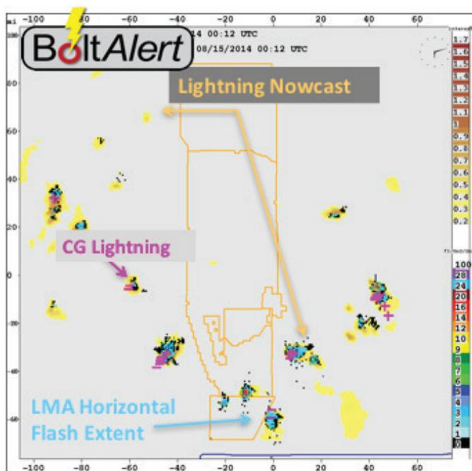
Lightning potential nowcast for an Army test range. Decision makers can use the information to safely evacuate personnel and protect sensitive equipment.
