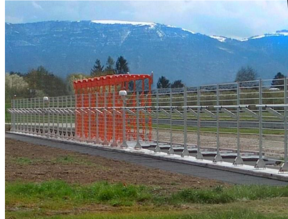
Our Cat III Model 201 Wide Aperture Localizer Antenna in Geneva, Switzerland
