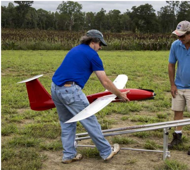
NASA engineers prepare to launch a remotely piloted aircraft during practice runs for an Unmanned Aircraft Systems Traffic Management test. (Image courtesy NASA.)
